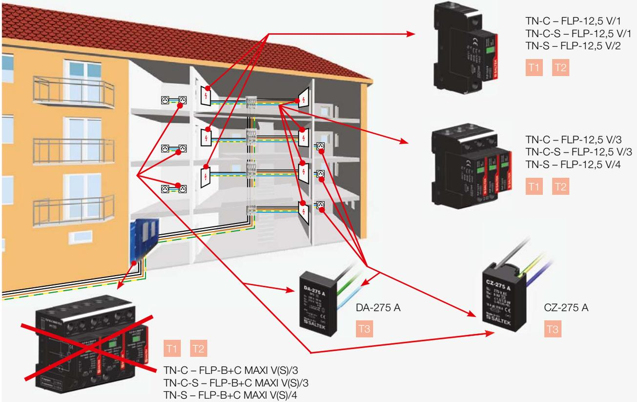
6 Blocks of flats with a cable connection with the possibility to install SPD type 1 in the unmeasured part
