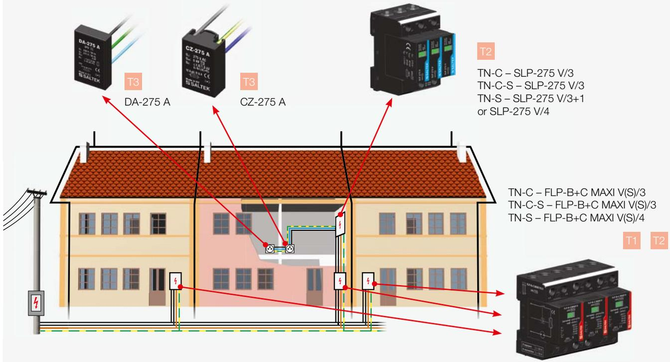
4 Terrace houses with a common down conductor and cable connection
