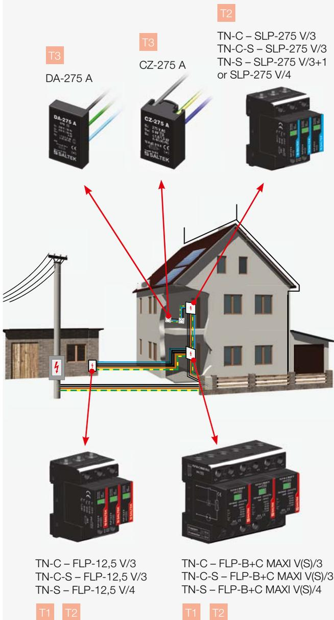
**2** A family house in a built-up area without a down conductor and cable connection
