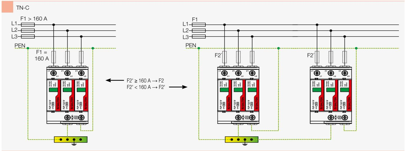
**5. Principles for positioning and connecting of lightning and surge arresters**
