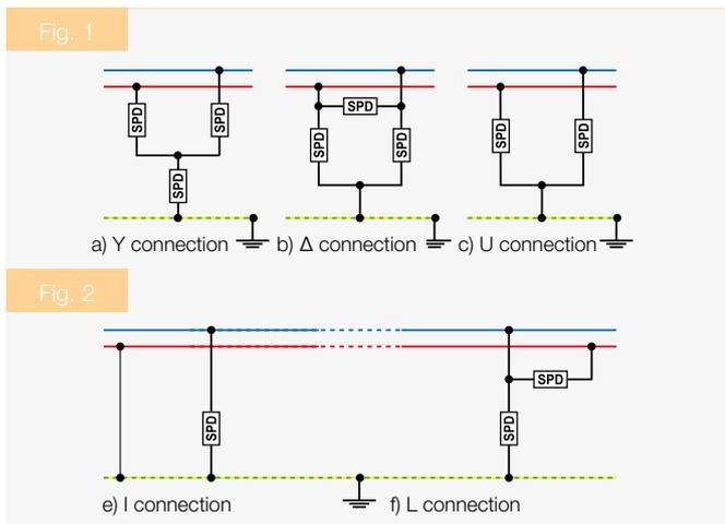
The DC side of the PV system can either be unearthed (insulated) or with one pole earthed. Figures 1 and 2 (see CLC/TS 50 539-12) show how SPDs on the DC side must be connected.
