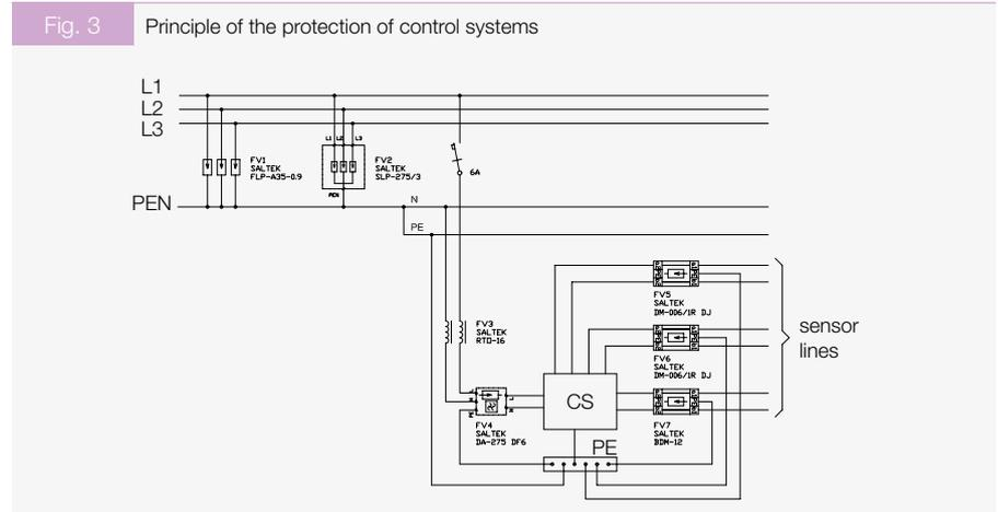
**The principle of placing the dataline protections**
